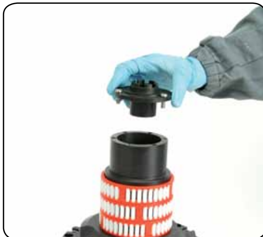
8. Remove the stripper arm housing n° 21
