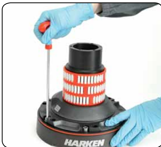
10. Unscrew the 6 hex screws n° 17 ( 20Nm/177 in-lb)
