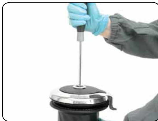
2. Unscrew the central screw ( \approx 2\text{Nm}/18\text{ in-lb} )
