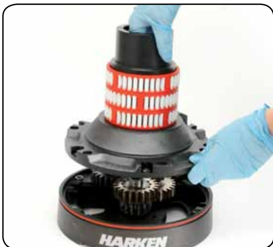
11. Remove the drum support n° 16
