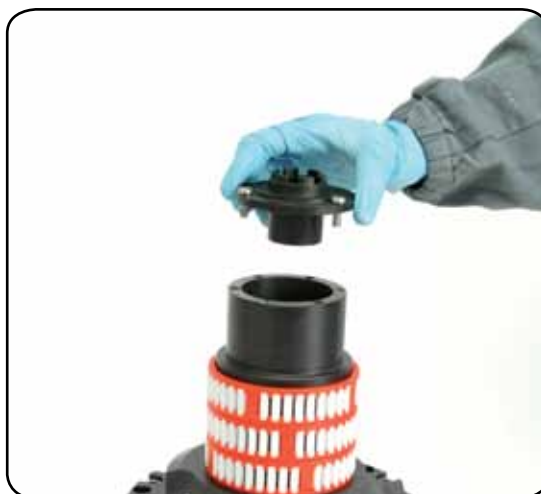
8. Remove the stripper arm housing n° 21
