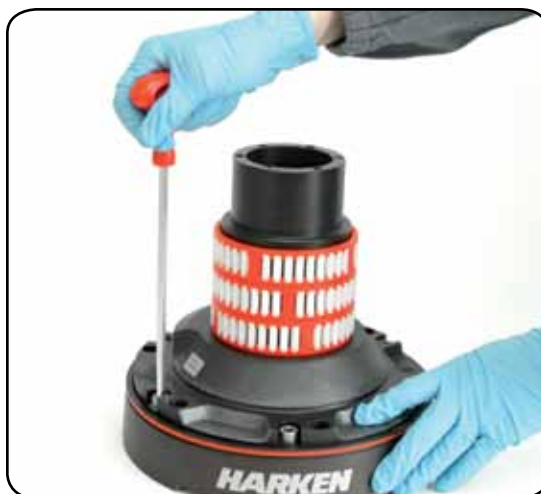
10. Unscrew the 6 hex screws n° 17 ( 20Nm/177 in-lb)
