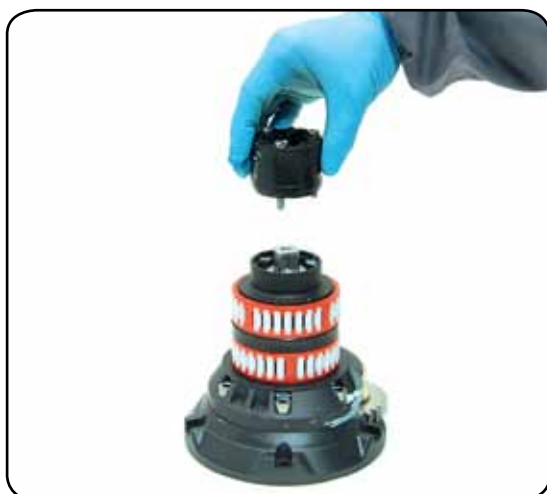
7. Completely unscrew the three screws n° 27 and remove the stripper arm support n°22
