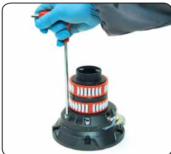
7. Completely unscrew the three screws n° 27 and remove the stripper arm support n°22
