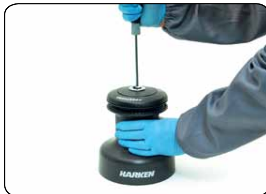
2. Unscrew the central screw ( \approx 2\text{Nm}/18\text{ in-lb} )
